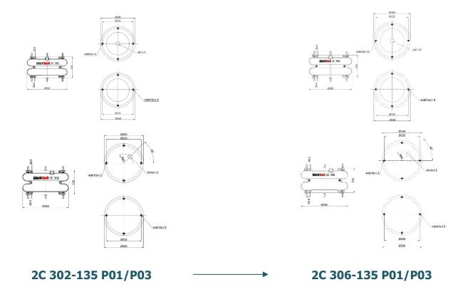
In order to to improve the efficiency of former Blacktech Versions **2C 302-135 P01** and **2C 302-135 P03**, we will switch to the revised versions **2C 306-135 P01** and **2C 306-135 P03**. In this case we will use instead of the metal ring, a steel ring consisting of a combination of many wires, which will be implemented during the vulcanization process. This will have a positive effect on the durability of our products.
